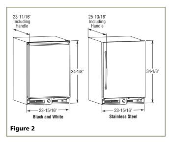
Please note that the unit has adjustable feet that can add one additional inch to height during leveling or to match adjacent cabinets (see **Figure 35** on **Page 14**).
